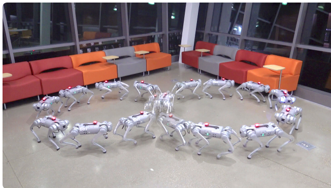
Fig. 1: With just a few lines of code in Python using PyPose, a quadruped robot can trace an \infty -shaped path.
