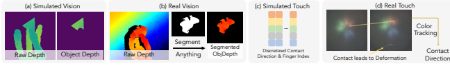
Fig. 3: Visuotactile information used in simulator and real-world. In simulation, we use the object’s foreground depth as the input. In real-world, to reduce the sim2real gap, we segment out the object’s depth map using Segment-Anything. For touch, we use discretized contact location in simulation provided by the simulator. In real-world, we parse the same information from temporal stream of tactile images.
