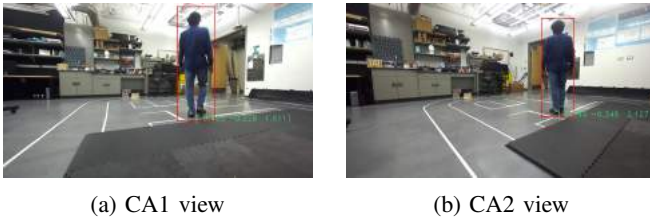
Fig. 5: Simultaneous Object detection and tracking of the pedestrian from two cameras having some relative orientation
