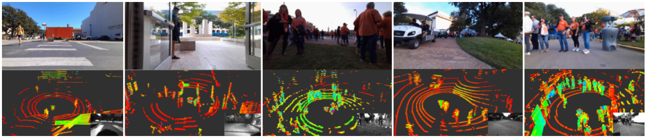
Fig. 2. Five example scenarios from SCAND showing the RGB image and below it the accompanying pointcloud with the monocular image. From left to right, the scenarios have the tags “Street Crossing”, “Narrow Doorway”, “Navigating Large Crowds”, “Vehicle Interaction”, and “Crossing Stationary Queue.”
