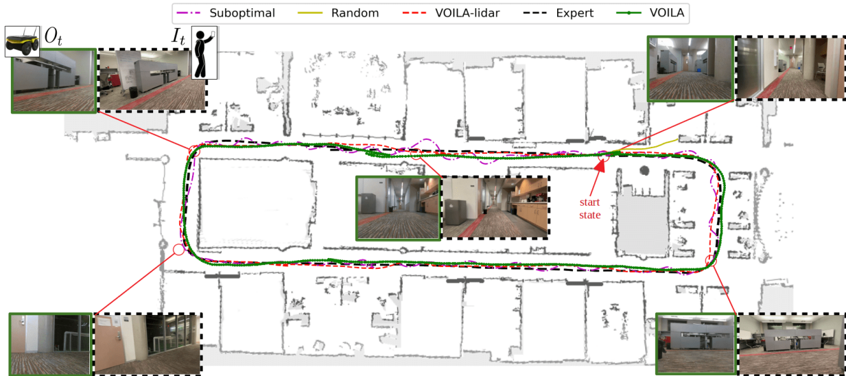
Fig. 1. Policy rollout trajectories of the VOILA agent (green) successfully imitating a demonstrated behavior (black) of patrolling a rectangular hallway clockwise. The demonstration consists of a video gathered by a human walking while using a handheld camera that is considerably higher than the robot’s camera (introducing significant viewpoint mismatch). We see that the VOILA agent is able to successfully imitate the expert demonstration even in the presence of this egocentric viewpoint mismatch.
