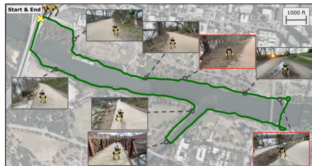
Fig. 5. A large-scale qualitative evaluation of STERLING on a 3-mile outdoor trail. STERLING features successfully complete the trail with only two manual interventions (shown in red).
