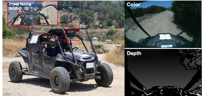
Fig. 1: Left: full vehicle with sensor suite, which consists of a high-resolution stereo camera and depth sensor. Right: RGB and depth images as viewed from the onboard camera during data collection and real-time inference.
