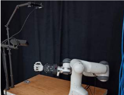
Fig. 4. View of the robot workspace. Two cameras are mounted on arms to enable visual perception. There is an ArUco marker [24] placed on the table to verify a constant position of the cameras.
