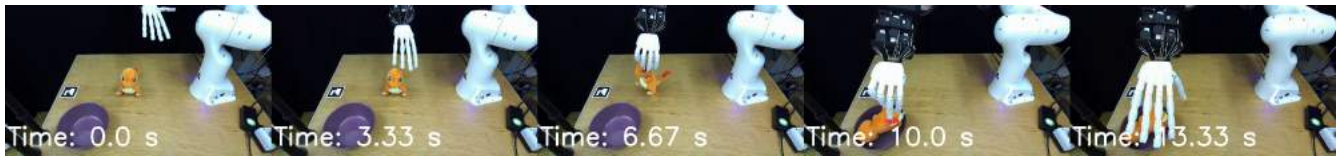
Fig. 6. A successful policy execution: the robot setup picks up the plush toy and places it into the bowl. The model can successfully fulfill this task from different initial robot states.
